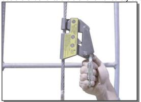
**Step 5:** Attach a CSA or an ANSI certified karabiner (according to the Jurisdiction) to the Slider. The attachment from the sternum D ring to the Slider should not exceed 0.15 M (6 in) in length. With the karabiner installed, the Slider cannot be removed from the cable. To ensure the Slider is functioning properly, pull down on karabiner to duplicate a fall arresting situation. Slider should grab the safety cable immediately.
