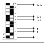
In this case, DIP SWITCH 1, 3, 4, 7, 8, 12 is put to ON, the result is 1+4+8+100+200+ 2,000=2313, the house No.2313
