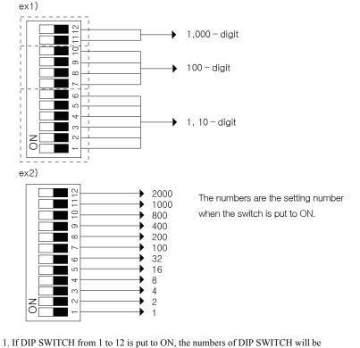
. If DIP SWITCH from 1 to 12 is put to ON, the numbers of DIP SWITCH will be summed up.
