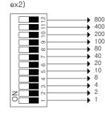
The numbers are the setting number when the switch is put to ON.
