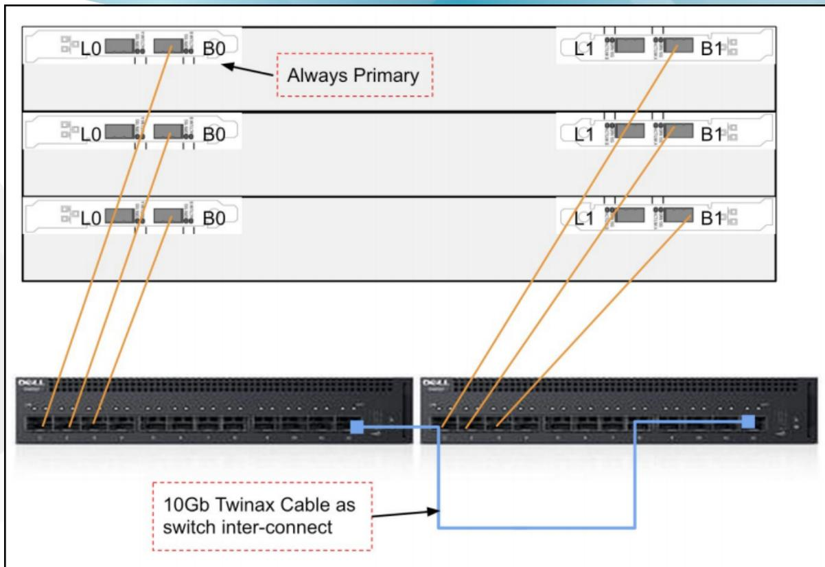
For both backplane and LAN networks on the cluster, the interfaces are in an Active/Passive bond, and not in a team or Active/Active bond.
