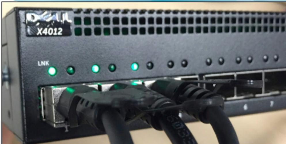
You can connect the power to the switch now, which will automatically power on. The default configuration for the X4012 is an isolated (default) single VLAN. The switch will not require any configuration as the goal is to have an isolated, non-routed network for node-to-node backplane communication only.
