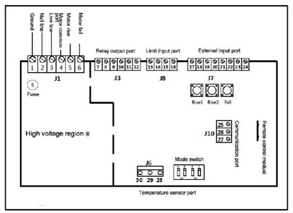
Wiring instruction: silk screen pedestal design number in bracket (symbol in correspondence with mainboard)
